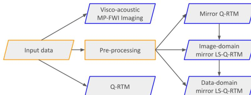
Figure 1: Processing and imaging flow chart. Items in the blue boxes are presented in this paper.
