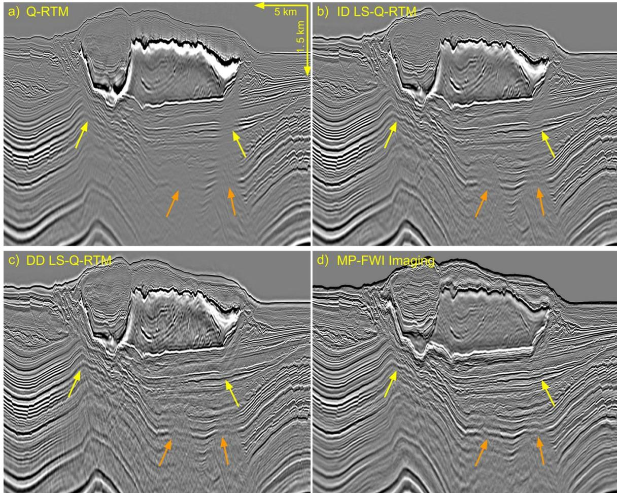
Figure 3: Mirror Q-RTM (a), image-domain LS-Q-RTM (b) and data-domain LS-Q-RTM (c) of the pre-processed down-going wavefield and MP-FWI imaging derived reflectivity (d).
