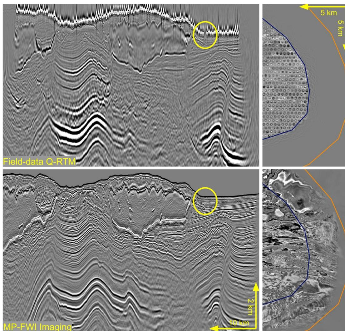
Figure 4: Section and shallow depth-slice tracking the water bottom through the Q-RTM (using up-going Green's functions) of the raw field data (top) and MP-FWI imaging reflectivity (bottom). The blue and orange lines describe the limit of the source and receiver carpets respectively.
