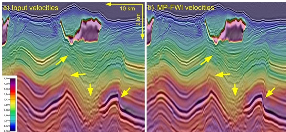
Figure 2: Input MP-FWI imaging velocity model co-rendered with a Q-RTM of pre-processed data (a) and output MP-FWI imaging velocity model co-rendered with a corresponding Q-RTM of pre-processed data (b).
