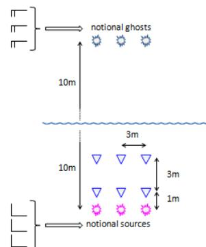
Figure 1 - The configuration of the simple test to demonstrate the derivation of notional ghost functions. The 3-gun array has 6 near field hydrophones. The notional sources are Dirac delta functions, the notional ghosts are a pairs of half amplitude negative Dirac delta functions.
