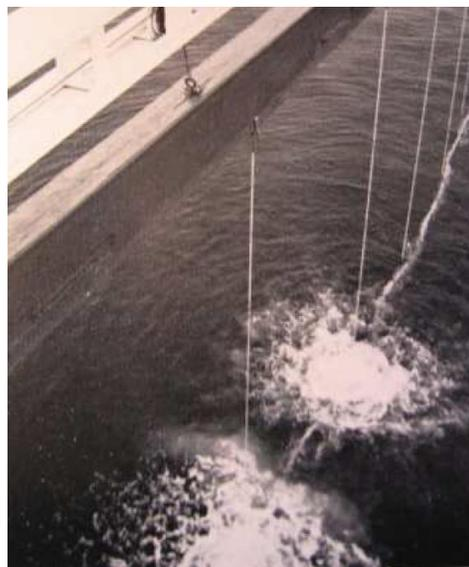
Figure 5 - The surface disruption known as the shot effect or spalling above two airguns. (from Hatton (2007) with permission).
