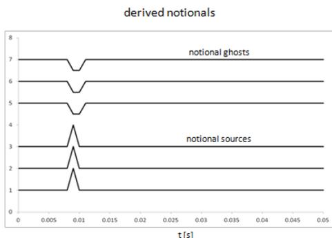
Figure 3 - The resulting notional ghosts and signatures derived from the hydrophone data. They correspond accurately to the notional functions used to generate the model data.
