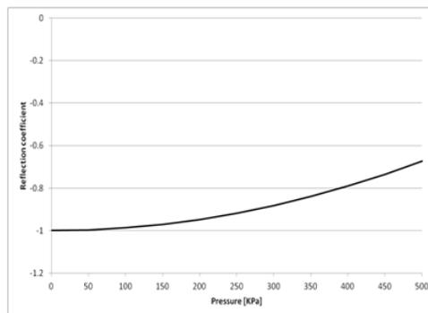
Figure 4 - Non-linear reflection coefficient at the free surface as a function of an incident pressure impulse.
