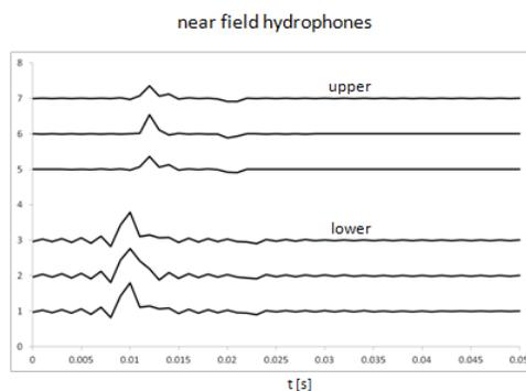
Figure 2 - The modelled near field hydrophone data for the simple 3-gun test in Figure 1.
