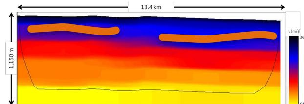
**Figure 5** Shows a slow-velocity layer defined by a velocity gradient from 386 m/s to 6333 m/s at 1067 meters depth derived directly from data in the Delaware Basin. We have inserted two high-velocity thin beds (orange) in different parts of the section.
