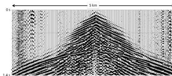
**Figure 1:** Shot record from a jebel in North Africa shows classic “Christmas-tree” pattern of refractor shingles consistent with a thick sequence of alternating high velocity and low velocity layers.
