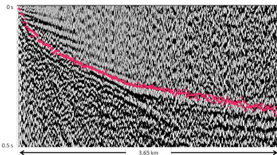
**Figure 4:** A shot displayed as a function of offset. Five distinct shingles can be seen on this record. The VwGradient is the smooth curve of picks starting at 0,0 on the left and transitioning smoothly to the deeper refractor about half-way across the record.
