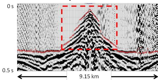
**Figure 2:** A single receiver line from a shot with LMO applied. Offset is plotted above the traces. Shingling appears on the inner offsets in the red box. The inner-offset shingling and the outer-offset deep refractor have been picked. Note the asymmetry of the shingle picks to either side of
