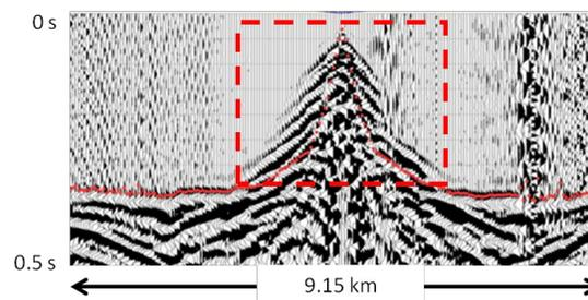
**Figure 3:** The same as Figure 2 except that instead of picking the shingled events, we have picked the VwGradient inside the box. The VwGradient is a continuous picking strategy that starts at (0,0) and connects smoothly with the deep refractor, seen here just outside the box.
