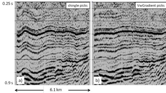
Figure 6 CMP stacks from the Midland Basin. a) Tomographic statics using only shingle picks. b) Tomographic statics using only vwGradient-derived turning ray picks.
