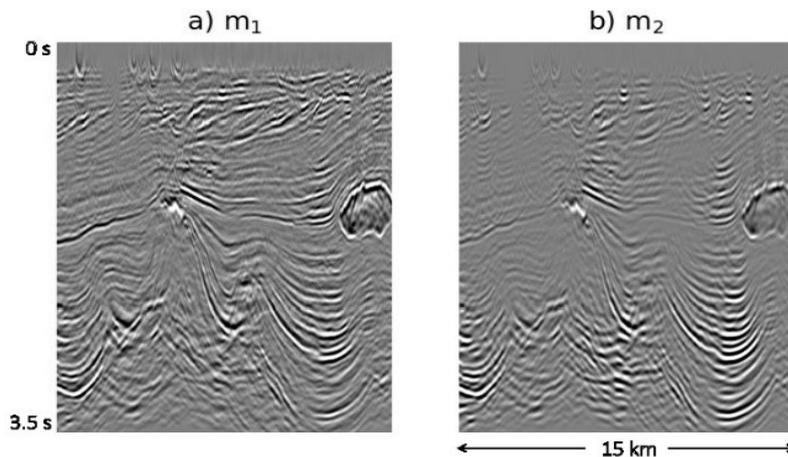
**Figure 2** a) First migrated image obtained using RTM; b) second migrated image obtained using remodeling and remigration exercise.
