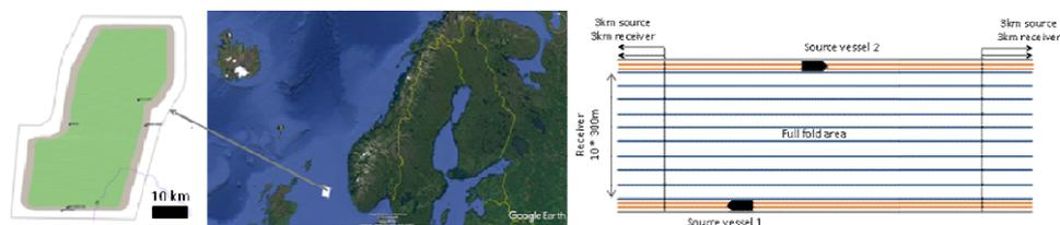
Figure 1 (top left) survey location and outline; (top right) initial two-vessel parallel acquisition pattern with receiver lines (blue) and source lines (orange). (Map courtesy of AGS)
