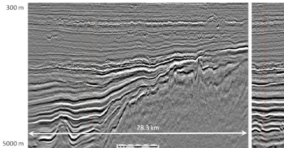
Figure 5 An inline and crossline through an up-going migrated stack volume. (Data courtesy of AGS)
