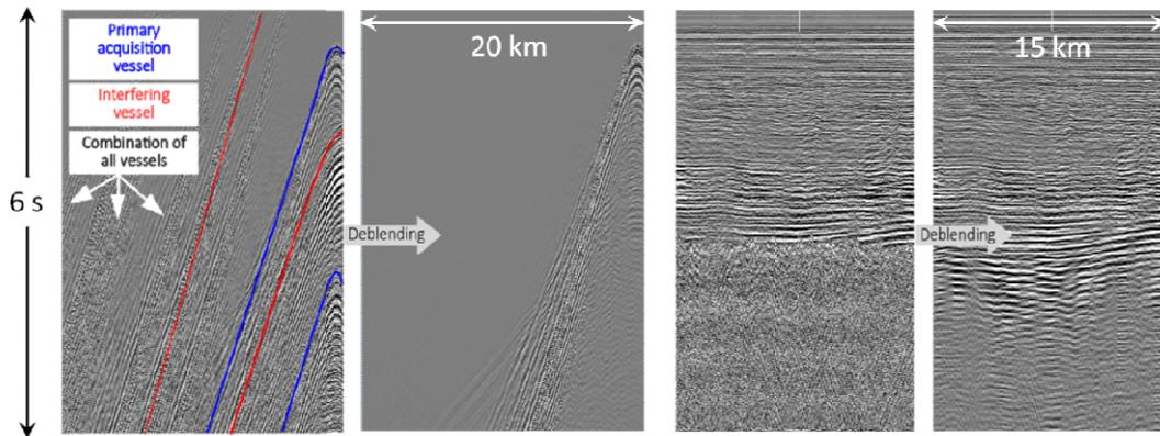
Figure 2 (left) shot gather before and after deblending. The overlapping energy from the primary acquisition vessel (shot 2 in blue) and the energy from the interfering vessel (red) have been successfully deblended. (right) Brute stack before and after deblending. The overlapping energy has been successfully deblended revealing deeper events. (Data courtesy of AGS)
