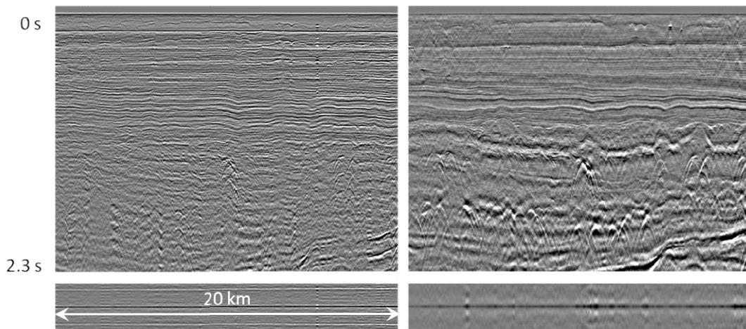
Figure 3 (left) stacked up-going wavefield with autocorrelation and (right) stacked U/D deconvolution with autocorrelation. (Data courtesy of AGS)
