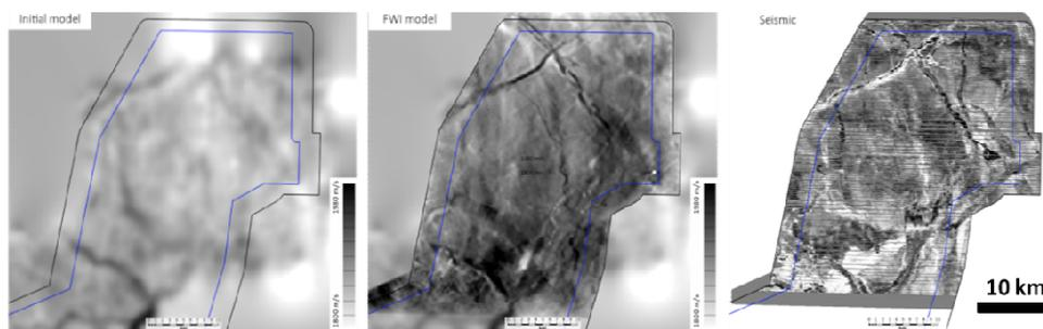
Figure 4 (left) Starting model for FWI and (middle) 5Hz FWI model. The shallow channels are resolved and match the structure on the migrated seismic stack (right). (Data courtesy of AGS)
