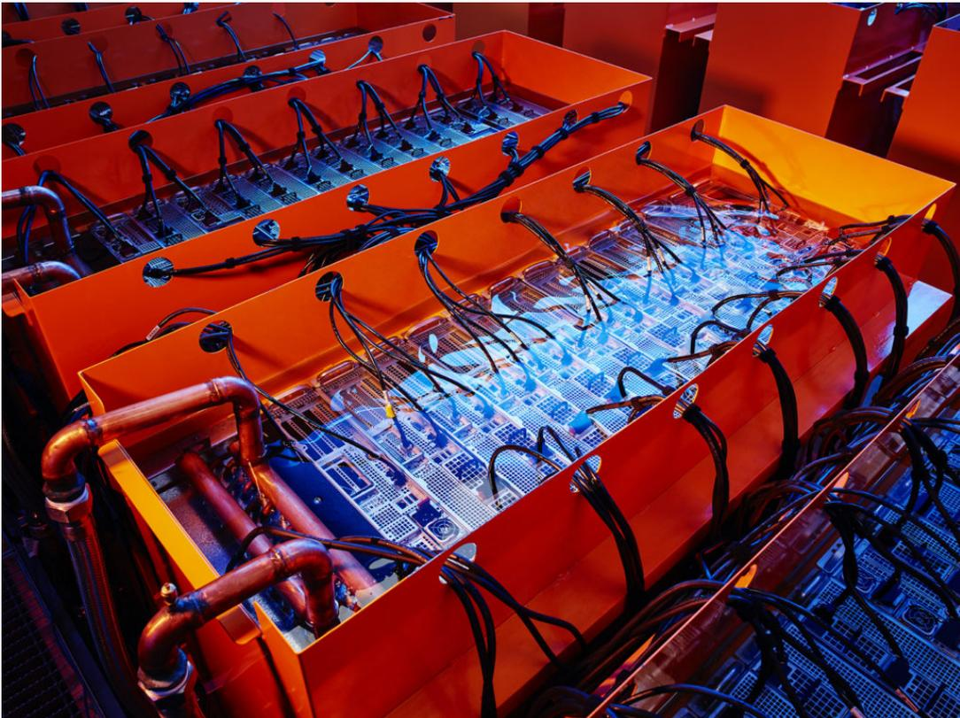
The huge application speedup was the result of DUG's HPCaaS. Seen here in DUG's immersion-cooled tanks located in West Perth. Image Credit: DUG.
