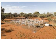
A 'tile' belonging to the Murchison Widefield Array (MWA) radio telescope.
