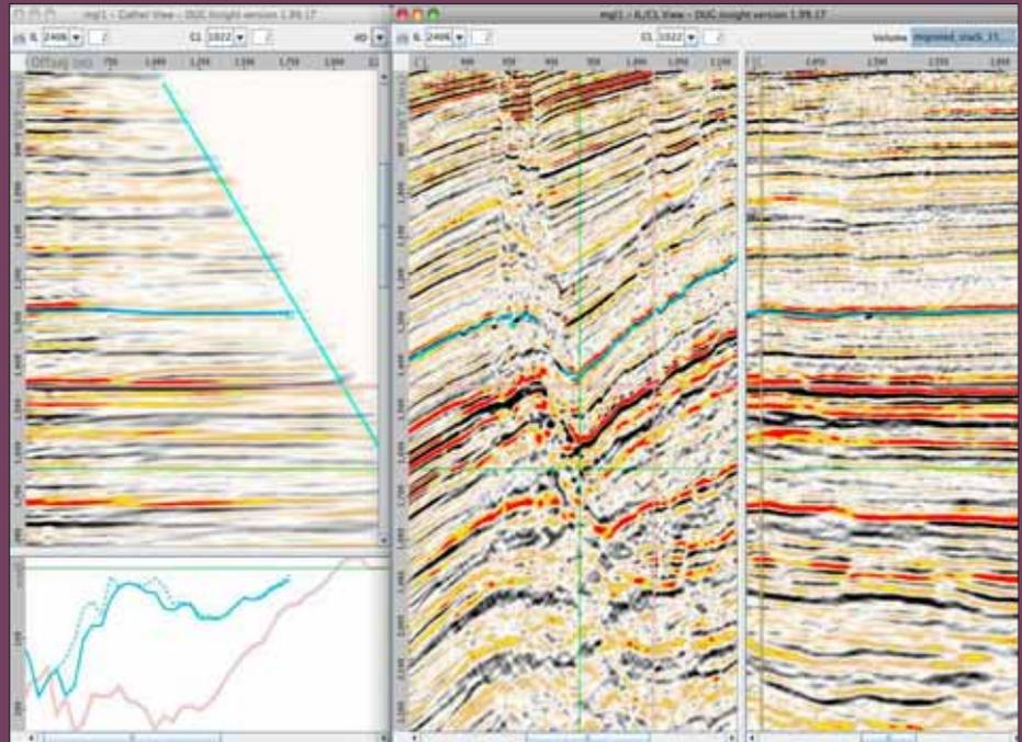
Fig. 1. A picked gather view together with the amplitude extractions across the gather and an il/cl view. This is an example of an integrated gather view from the DUG Insight software.
