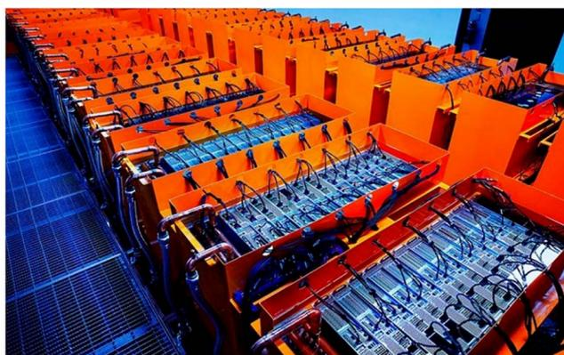
“Bruce,” DUG’s Perth cluster, comprised of KNL nodes, totaling 20 single-precision petaflops. The “Bubba” tanks currently being installed at the Houston Skybox facility will look similar to these. Photo provided by DUG.
