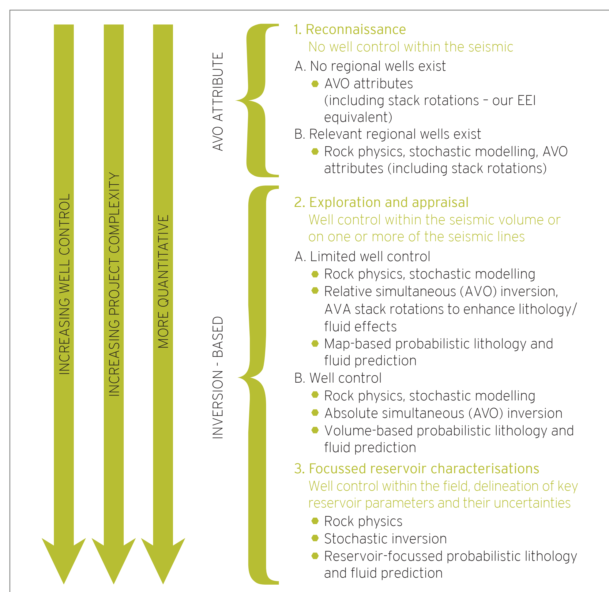
Figure 1. High level road map of range of QI options available for seismic reservoir characterisation.
