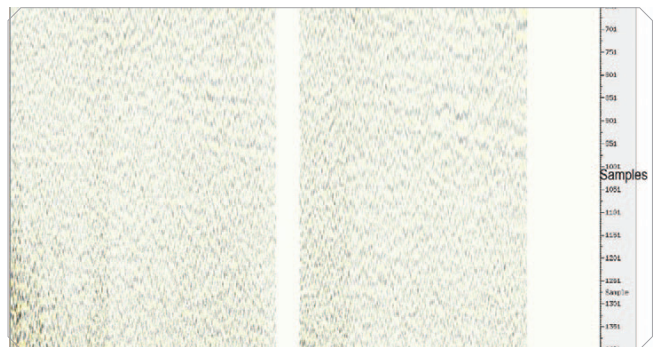
FIGURE 10 Vibroseis to hydrophone, after noise removal.
