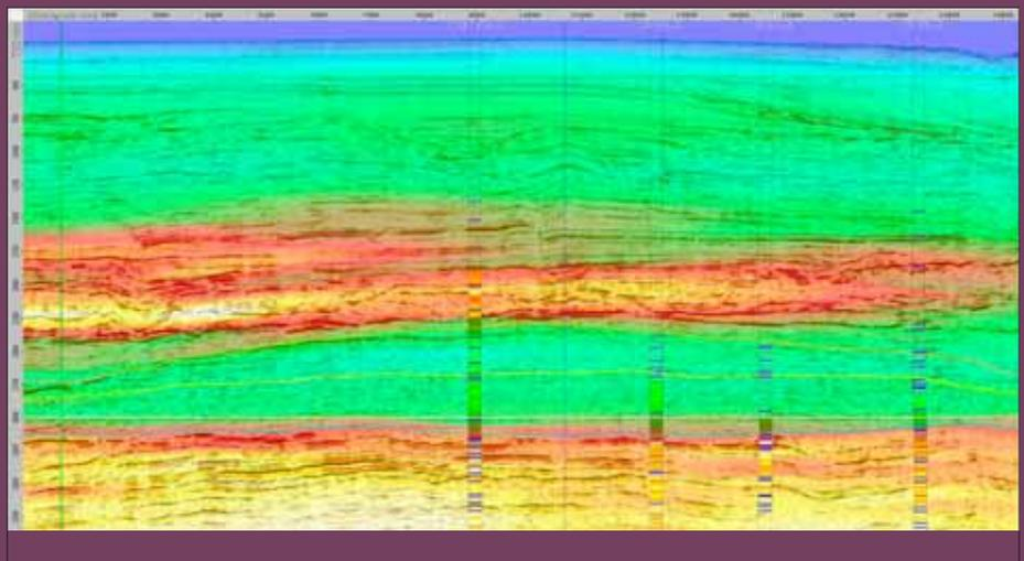
Fig. 5. An arbline view with a full stack co-rendered with a velocity field. The display also has velocity logs posted at the well trajectory positions.
