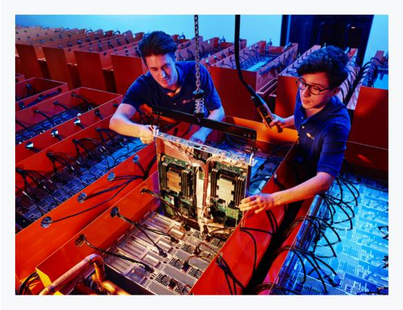
The huge application speedup was the result of DUG's HPCaaS. Seen here in DUG's immersion-cooled tanks located in West Perth. Image Credit: DUG.
