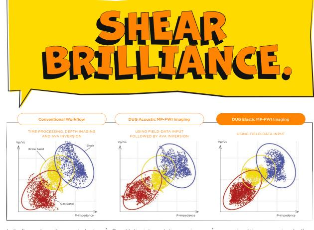
In the figure above, three equivalent crossplots of elastic rock properties are compared. The ellipses indicate the expected distribution of the labelled lithology and fluid combinations from statistical rock physics analyses of well log data.
