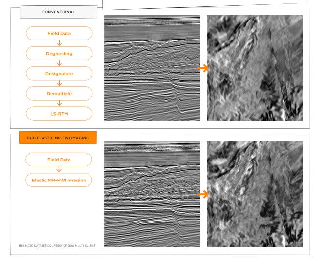
Comparison of the reflectivity derived with DUG Elastic MP-FWI Imaging using raw field data, versus a conventional LS-RTM workflow using extensively pre-processed input. This legacy dataset was acquired in 2006 on the Australian North West Shelf. This region contains rapidly changing shallow velocity variations due to localised channel features and carbonates.
