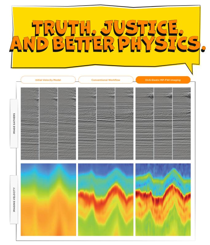
The Earth is inherently elastic. As data processing has advanced to better honour physics, we have continually refined our ability to understand the subsurface. Here, velocity model updates generated using a conventional workflow and DUG Elastic MP-FWI Imaging were evaluated using a Kirchhoff pre-stack depth migration (KpreSDM), using the fully pre-processed data as input. The figure above compares common-offset-vector KpreSDM snail gathers using the initial velocity model (left), the
