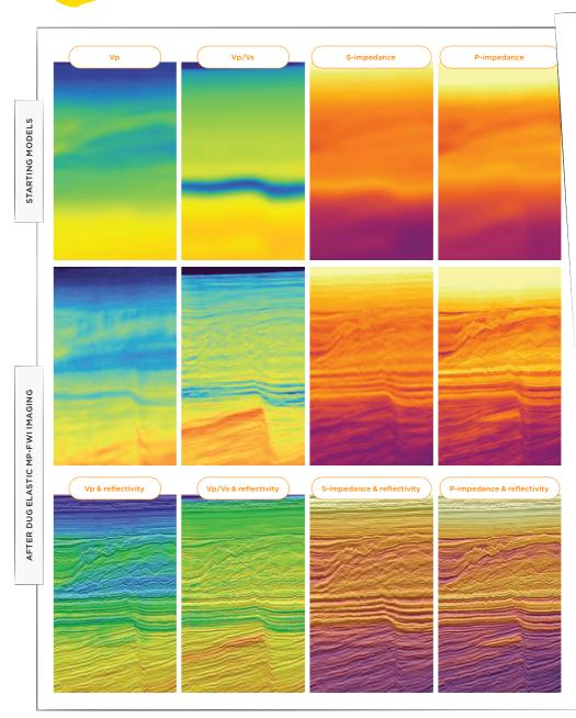
DUG Elastic MP-FWI Imaging enables simultaneous inversion of reflectivity (3-component, directional, horizontal), P-wave velocity, S-wave velocity, density, P-impedance and S-impedance, providing quantitative interpretation-ready outputs of the highest resolution and amplitude fidelity — using field data input. Simply fantastic!
